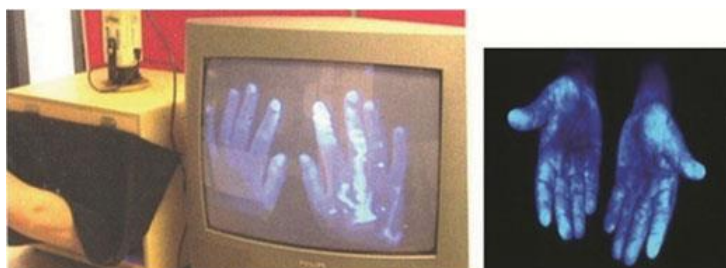
Figure 4: A portable system for detection of the tracers on the skin and surfaces 18
