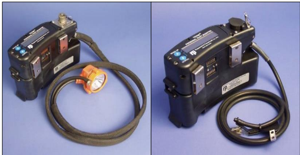
Figure 3.12 Series 3600 monitor with integrated cap-lamp for mining and Series 3700 monitor for general occupational hygiene monitoring
