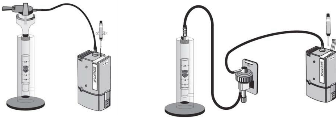
Figure 3.8 Sampling Train for Pump Calibration 2
