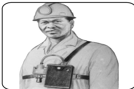
Figure 3.7 Early Model Personal Respirable Dust Sampler Attached via a Harness
